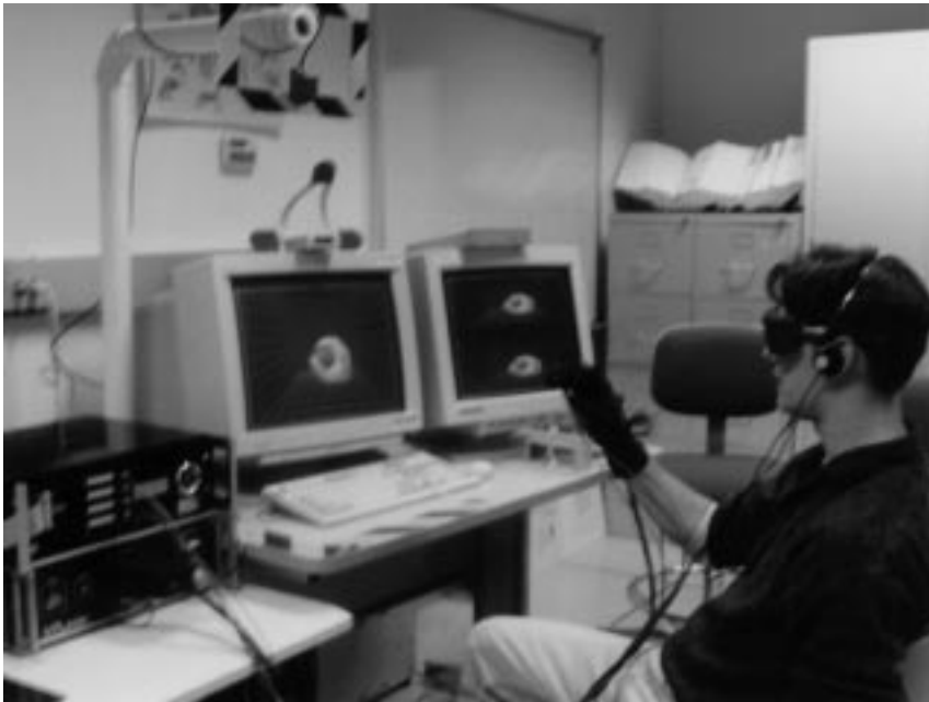
Figure 9.6: Using the force feedback data glove and simulated sound, a virtual handball game is played with the computer. The operator wears glasses to perceive the display in 3-dimensions. Under program control the resilience of the ball can be varied, as well as its dynamic properties. This same facility is being used in medical experiments aimed to train endoscopic surgery and joint palpation.
