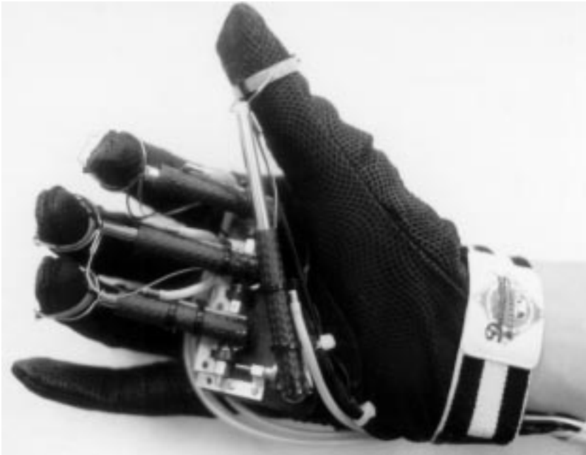
Figure 9.5: CAIP's force feedback transducers for a data glove are single-axis pneumatic thrusters, capable of sensing finger force or, conversely, of applying programmed force sequences to the hand. Joint motion is sensed by optical fibers in the glove, and hand position is measured magnetically by the Polhemus sensor.
